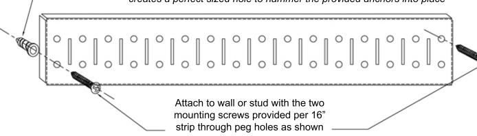
Warning: Do not over tighten mounting screws or risk damaging the panel face
