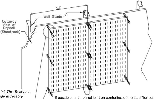
Quick Tip: To span a single accessory across multiple panels, a penny's thickness between the panels creates the perfect spacing. Note, this is not required for any Wall Control accessory
